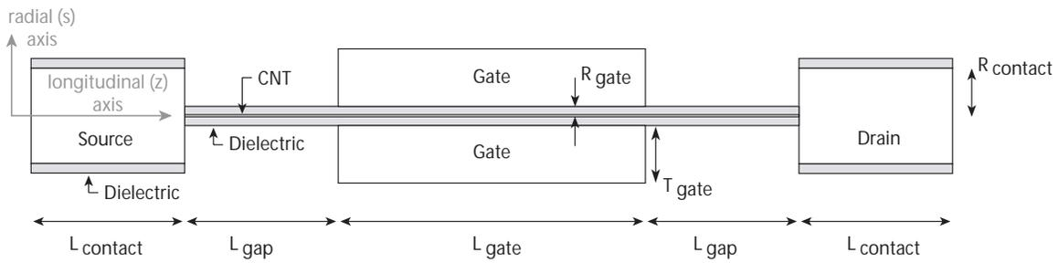
Figure 1: PG-CNFET device structure.
