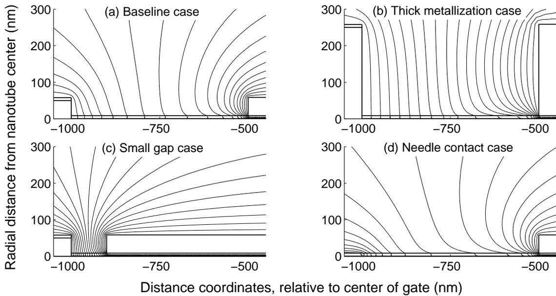
Figure 2: Equipotential plots for the PG-CNFETs listed in the first four rows of Table 1 for  $V_{GS} = 0.5$  V. The equipotential contours are at intervals of 24 mV. The source is on the left, and the gate is on the right. The dielectric between the source and gate is visible at the bottom of each figure, but the nanotube is too narrow to be discernible.
