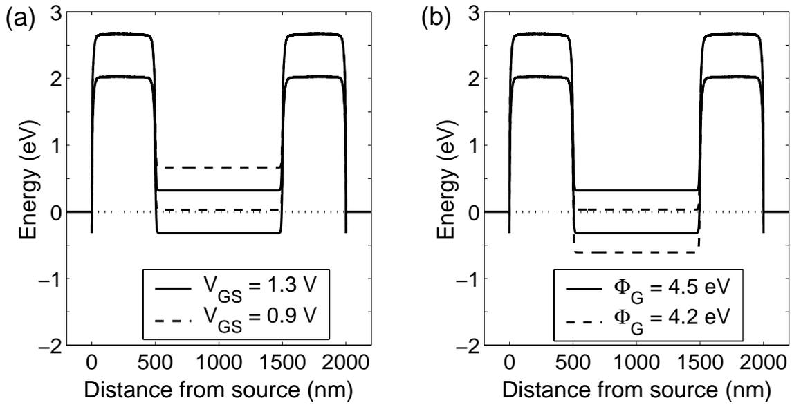
Figure 5: Energy-band diagrams for the PG-CNFET of Ref. [5]. (a) Operating as a  $p$ -type device, being in the ON state at  $V_{GS} = 0.9$  V, and the OFF state at 1.3 V. (b) Operating as an  $n$ -type device at  $V_{GS} = 1.3$  V, and being turned ON with a gate work function change from 4.5 to 4.2 eV.
