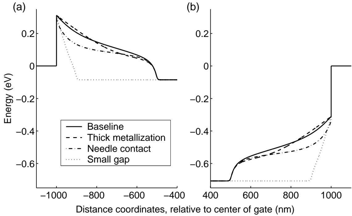
Figure 3: Energy-band diagrams for the devices described in the first four rows of Table 1. The energy is measured with respect to the Fermi level at the end contacts. (a) The conduction-band profile at the source end. (b) The valence-band profile at the drain end.
