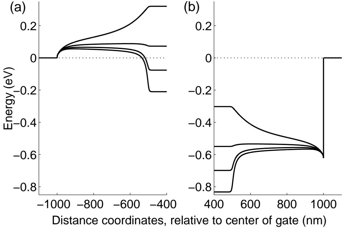
Figure 4: Energy-band diagrams for the low-work-function device described in the fifth row of Table 1. The energy is measured with respect to the Fermi level at the end contacts (dotted line). The parameter is  $V_{GS}$ , and it ranges from 0 (top line) to 0.75 V (bottom line) in increments of 0.25 V. (a) The conduction-band profile at the source end. (b) The valence-band profile at the drain end.
